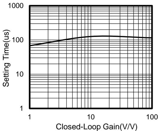
Figure 21. Setting Time vs Closed-loop Gain
