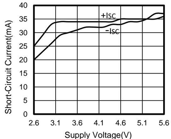
Figure 12. Power Supply Voltage vs Short Circuit Current
