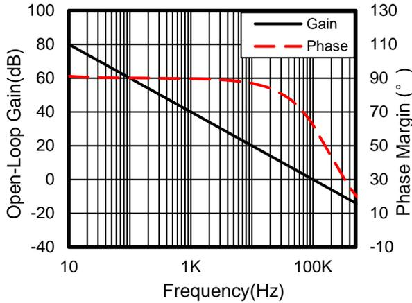
Figure 1. Open-loop Gain and Phase vs Frequency
