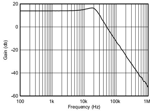
Figure 27. Low-pass filter transfer function
