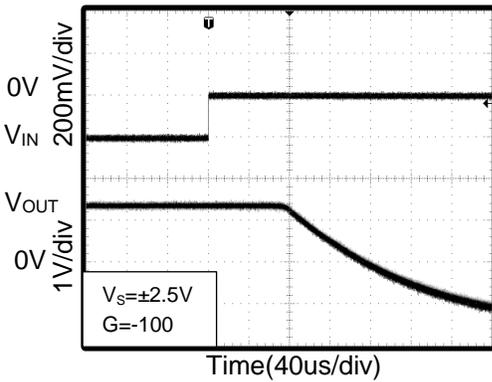
Figure 13. Positive Overload Recovery
