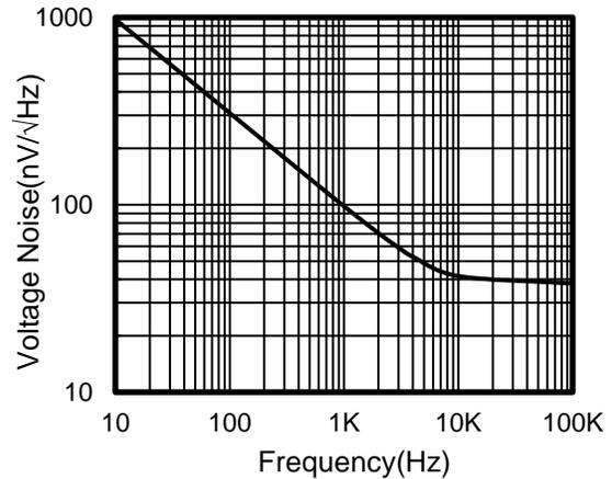
Figure 2. Input Voltage Noise Spectral Density vs Frequency
