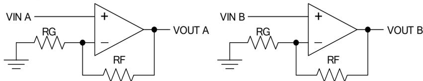
**Figure 28. Schematic Representation**
