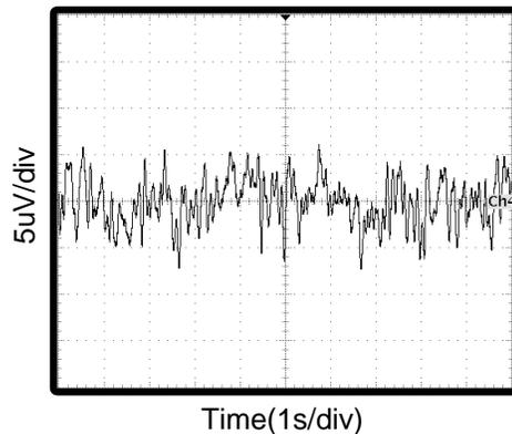
Figure 10. 0.1Hz to 10Hz Input Voltage Noise
